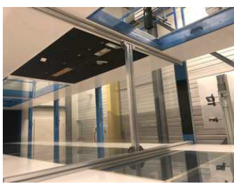
Figure 1: (a) photography of the experimental configuration of the double parallel bars in the LMFL wind tunnel. The flow is coming from the right. (b) Horizontal kinetic energy per unit mass computed from velocity measured by PIV in the wake behind the two parallel bars at the beginning of the measurement run. (c) Same field, 250s later.
